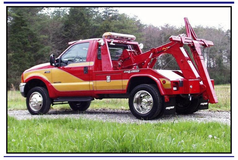
**The Challenger Express** brings hydraulic auto loads to a higher level with features that include extended reach for easy vision and hook-up; newly designed crossbar approach plate; a 3" pivot pin and a roller guided hose tracking system for less maintenance and downtime. Check out the features and find out how the **Challenger Express** can help increase your profits, not your downtime.
