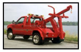
This Challenger 4311 Express, shown here with the standard heavy duty steel body and the Challenger 4312 Express, provide the operator with a hydraulic extendable recovery boom.
