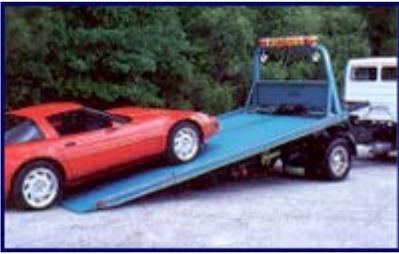
After the vehicles' front wheels are on the carrier, the bed can then be leveled out and the cable guide removed, allowing the vehicle to overcome the second clearance problem on the forward section of the deck. This problem is encountered on carrier decks with the rear section permanently angled.
