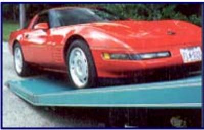
With the front wheels now on the front section of the deck, the operator is able to angle the rear section a second time. This is not necessary except in cases where you have low clearance on the rear of the vehicle such as low rear spoilers, exhaust pipes or low bumpers.
