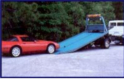
The camlocks are released and the bed tilted allowing the rear section of the deck to hinge to a load angle of 6°. A removable cable guide is inserted into the bed so the cable is held low to the bed and away from the vehicles' spoiler or air dams.
