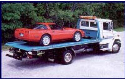
With the vehicle tires fully on the carrier, the deck may be leveled out again and the loading process completed. The camlocks are engaged so that the rear section is locked in place while you secure the vehicle.
