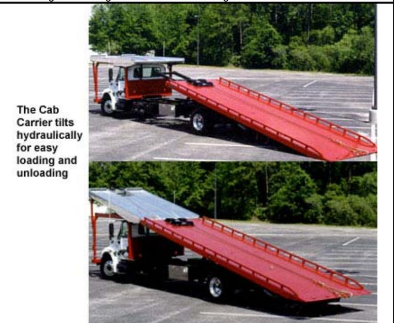
The Cab Carrier tilts hydraulically for easy loading and unloading
